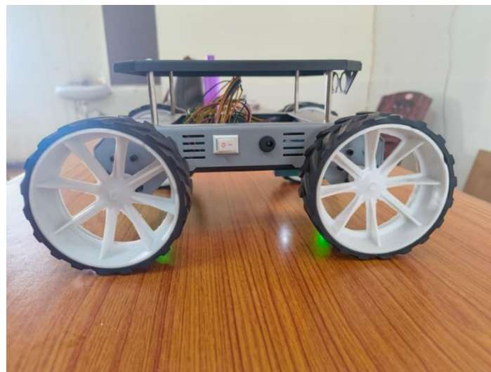
Fig. 4: Side View of Four-Wheeled Mobile Robot Platform with Power Switch and Integrated Electronics
