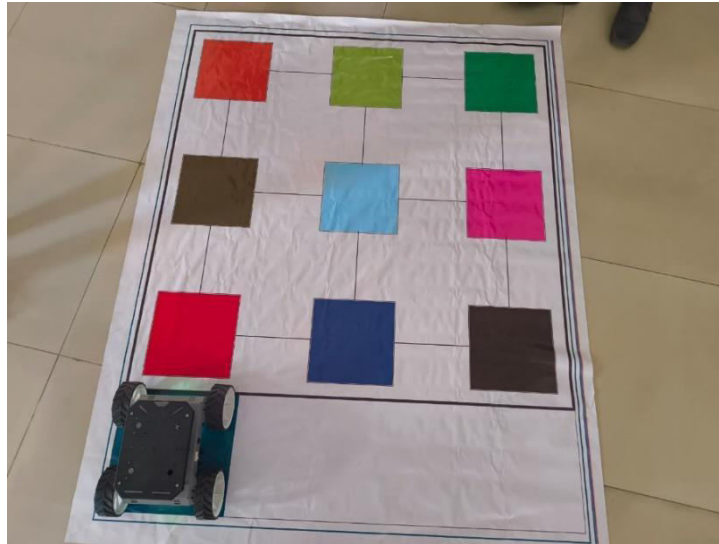
Fig. 5: Experimental Setup of Mobile Robot on Grid-Based Colored Navigation Mat
